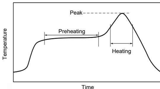
For soldering (Example : Sn/Pb)
